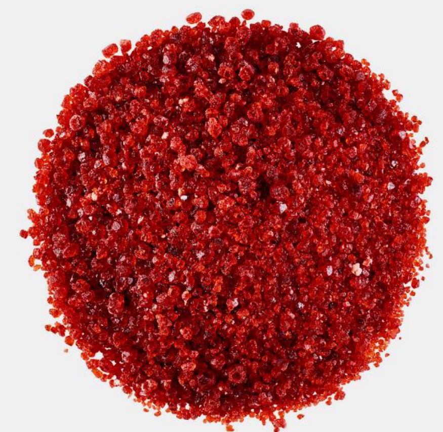
Cobalt sulfate crystals from nodules
